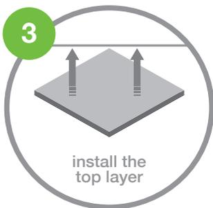
**Install the top (constrained) layer.** Peel off the second release liner of the DIS8 and apply a top layer such as steel plate or plasterboard to the damping sheet. Apply firm hand pressure or use a roller to push the top layer onto the DIS8.
