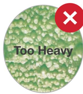
Representation of a **TOO HEAVY** pattern as sprayed too slowly with an improperly adjusted gun. The pattern shows significant bubbling and agglomeration that can lead to solvent entrapment and poor coverage.
