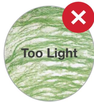
Representation of a **TOO LIGHT** pattern as sprayed too quickly across the substrate. The pattern shows significant voids and indicates little adhesive disposition.
