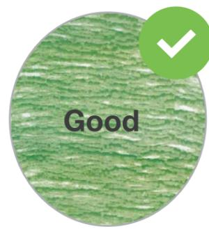
Representation of a **GOOD** pattern as sprayed from a properly adjusted gun. The pattern should have at least 90% of the surface covered with at least 2.5 grams of dry adhesive deposited per square foot of substrate.
