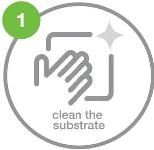
**Clean the substrate surface** with Megasorber AC5, acetone or similar. The surface must be dry, free of oil, dust, grease, rust and other contaminants.
