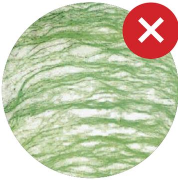
Representation of a **TOO LIGHT** pattern as sprayed too quickly across the substrate. The pattern shows significant voids and indicates little adhesive disposition
