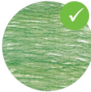
Representation of a **GOOD** pattern as sprayed from a properly adjusted gun. The pattern should have at least 90% of the surface covered with at least 2.5 grams of dry adhesive deposited per square foot of substrate
