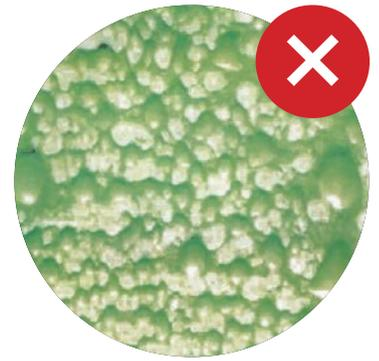
Representation of a **TOO HEAVY** pattern as sprayed too slowly with an improperly adjusted gun. The pattern shows significant bubbling and agglomeration that can lead to solvent entrapment and poor coverage.
